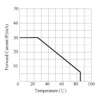
FORWARD CURRENT VS. AMBIENT TEMPERATURE
