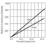
FORWARD CURRENT VS. LUMINOUS INTENSITY
