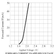
FORWARD CURRENT VS.APPLIED VOLTAGE
