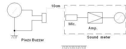
Input Signal 12V DC Test Distance 10cm
